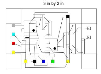
Current sensor is "brick transformer" with primary cut out and replaced with several turns of 14 AWG wire in series with black wire on supply to washer. This circuit can detect load currents between about 2.5 and 20 amps
